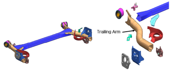
Fig. 10. Schematic drawing of a trailing arm.
