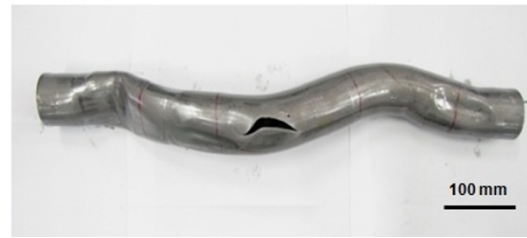
Fig. 13. Cracking in hydroformed trailing arm.
