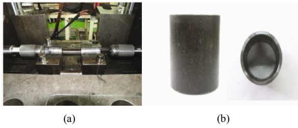
Fig. 6. (a) Die set for free bulging test; (b) restrictive ring.
