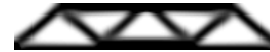
Fig. 4. The initial optimal topology of the MBB beam using the proposed approach with 180 \times 30 mesh.
