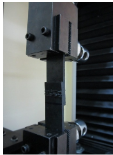
Fig. 6. Specimen and fixture during TSS test.
