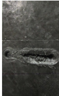
Fig. 1. Weld joint obtained at RS = 630 rpm, WS = 12 mm/min and TA = 0°.
