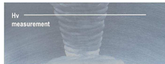
Fig. 5. OM structure of the Alloy 617 weldments.
