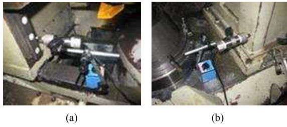
Fig. 11. Grating displacement sensor Installation of thermal deformation: (a) Large column bottom; (b) Small column bottom.
