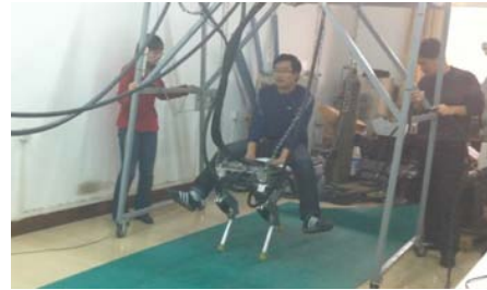
Fig. 13. Scaif-1 trotting with 80 kg payload at 0.4 m/s.
