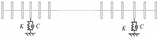
Fig. 7. Transfer matrix model of bearing-rotor system.
