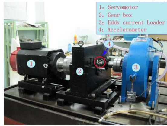
Fig. 16. Open power flow experimental system.
