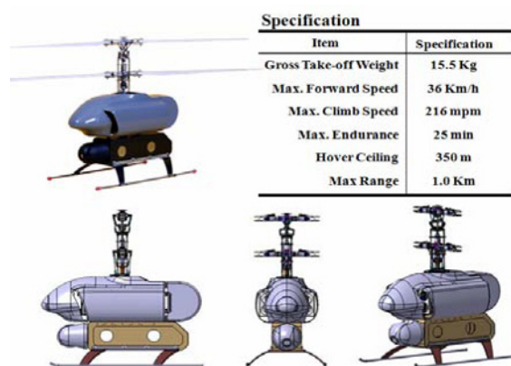
Fig. 1. Configuration of a coaxial helicopter.
