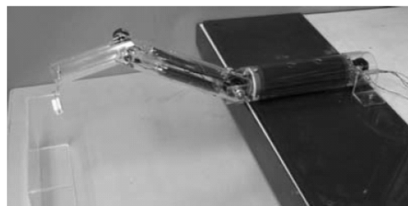
Fig. 10. Robot arm using electrostatic motors.
