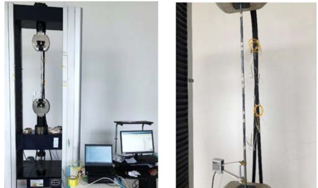
Fig. 8. Static Tensile Test of HSW-FBG Sensors
