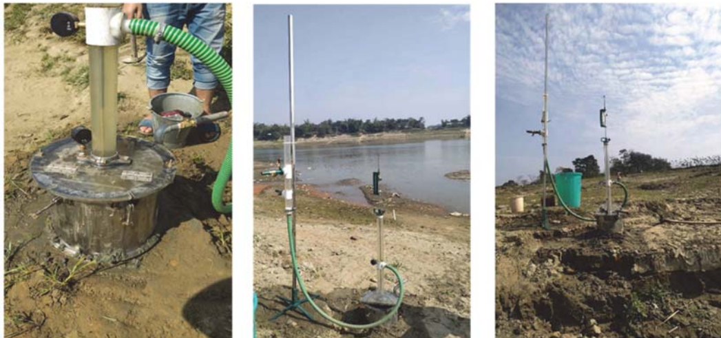
Fig. 3. Examples of Submerged JET Test Being Performed in the Bank of Barak River
