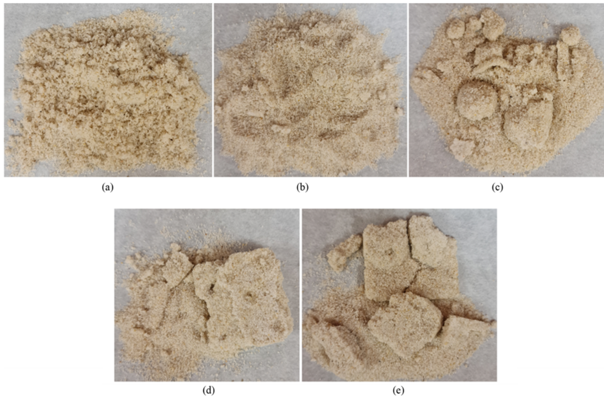
Fig. 5. A Representative Example of Specimen's Shape after Shearing for Each Method of EICP Solution Application: (a) Spray Method, (b) Mix-&-Compact Method, (c) Percolation Method, (d) Injection Method, Specimen 1, (e) Injection Method, Specimen 2
