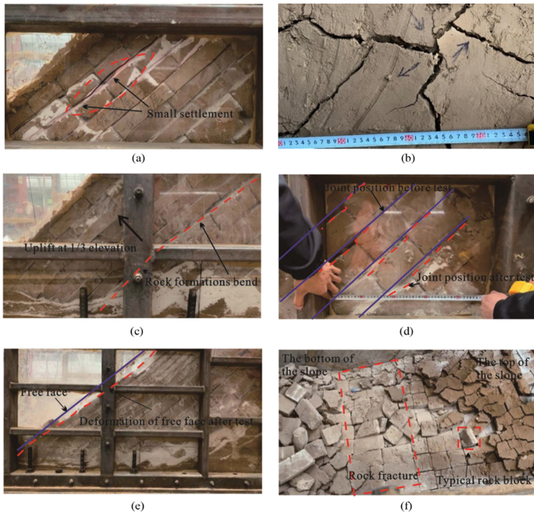
Fig. 18. Failure Process of Slope Model: (a) Small Settlement of Rock Layer, (b) Uplift at the 1/4 Height, (c) Rock Layer Bend at the Slope Toe, (d) Thick Rock Fracture, (e) Fallen Thin Hard Rock Layer, (f) Overall Condition of Slope Surface Fragmentation
