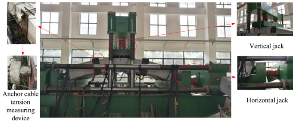
Fig. 5. Local Prototype Structure Loading System
