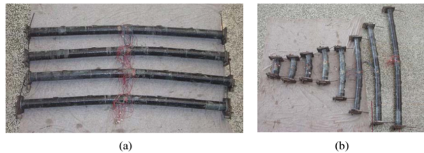
Fig. 5. Several Specimens after Testing: (a) Specimens of \lambda = 90 , (b) Specimens of e = 1.3
