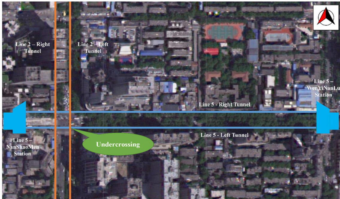
Fig. 9. The Plan View of No. 5 Shield Tunnel Under-Crossing No. 2 Subway in Xi'
