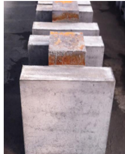
Fig. 6. Finished Products of the Push-Out Test Specimens
