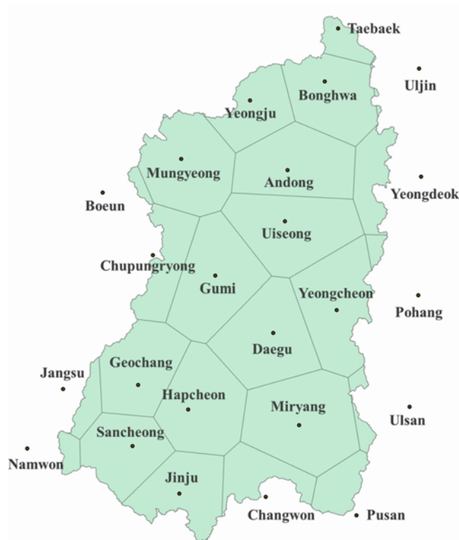
Fig. 4. Meteorological Stations and Thiessen Network
