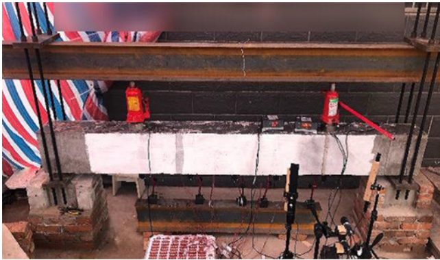
Fig. 11. Loading Procedure of the Test Beams
