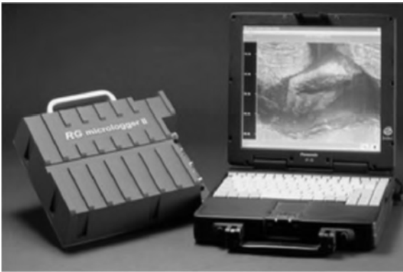
Fig. 2. High Resolution Acoustic Televiewer
