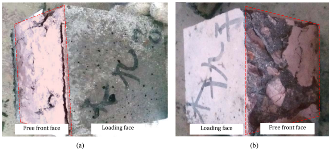
Fig. 4. The Comparison of Failure Patterns in Admixtures: (a) 15SF-1STF, (b) RF-15SF-0STF in Compressive Strength Test
