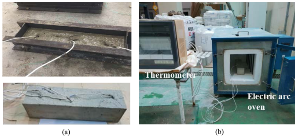
Fig. 1. Set-Up of Conducting the Chamber Test: (a) Concrete Specimen, (b) Experiment Equipment
