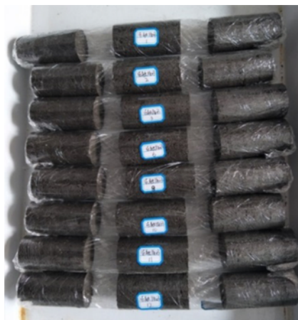
Fig. 2. Various Modified Expansive Soil Specimens Prepared
