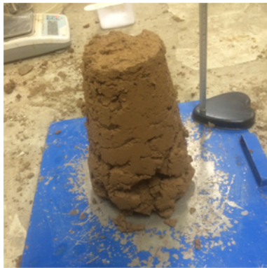
Fig. 7. Soil Sample with Water Content of 10 % (FIR = 88%)
