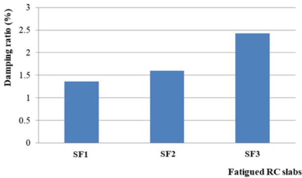
Fig. 9. Damping Ratios of Fatigued RC Slabs at Lower Mode
