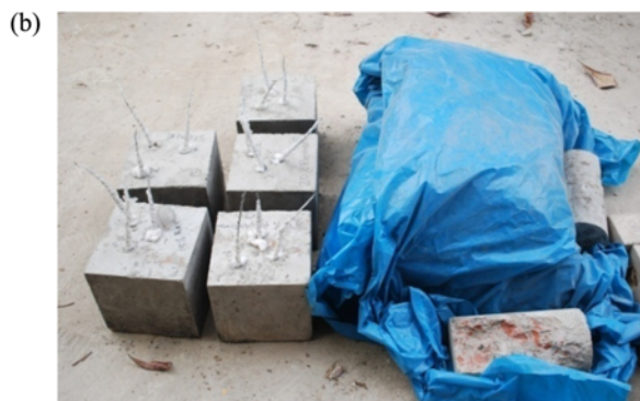
Fig. 4. Internal RH Measurement: (a) Schematic Diagram, (b) Cubes under WP and WOP Conditions
