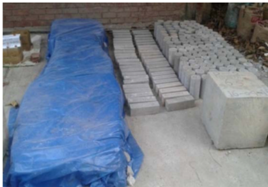
Fig. 3. Samples Were Kept Outside with (WP) and without (WOP) Polythene Cover
