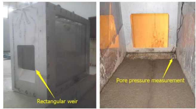
Fig. 5. Layout of the Pore Pressure Measurement
