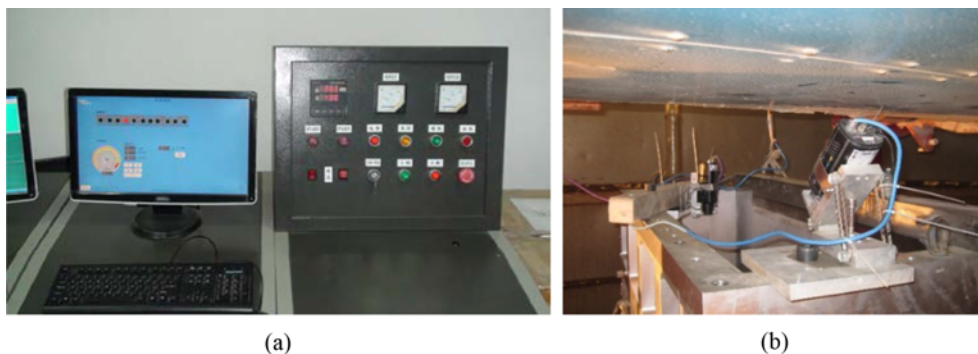
Fig. 6. Data Acquisition System: (a) The Industrial Personal Computer, (b) Cameras Placed on the Model Box
