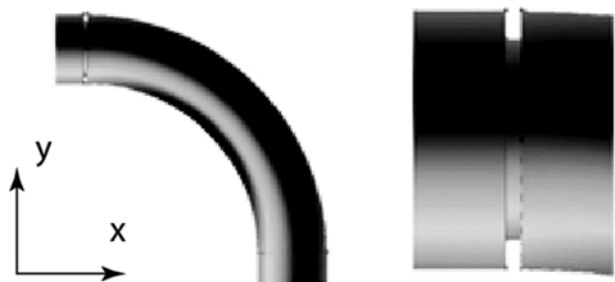
Fig. 3. A 40% Obstruction Placed at the Leading Edge of the Bend
