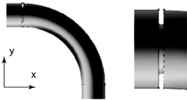
Fig. 4. A 60% Obstruction Placed at the Leading Edge of the Bend
