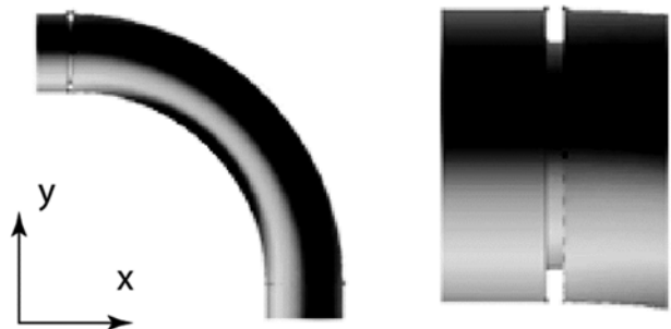
Fig. 2. A 20% Obstruction Placed at the Leading Edge of the Bend
