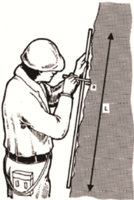
Fig. 7. Method of Measuring Joint Trace Amplitude (Morelli, 2014)
