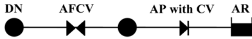
DN: Demand Node; AFCV: Artificial Flow Control Valve; AP with CV: Artificial Pipe with Check Valve; AR: Artificial Reservoir
