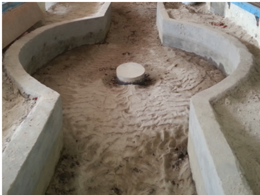
Fig. 1. Showing the Model of Braided Bar Constructed in a River Engineering Laboratory IIT Roorkee
