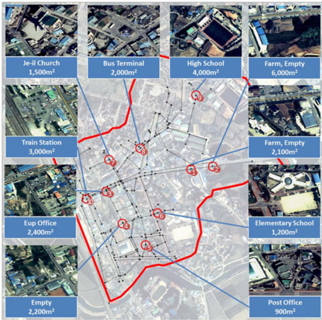
Fig. 6. Potential Locations for Storage Facility Construction
