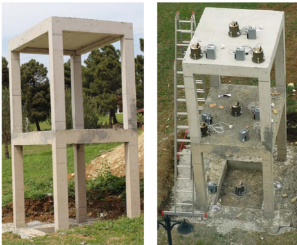
Fig. 6. Accelerometers Location on the Test Structure (1 st configuration scheme)
