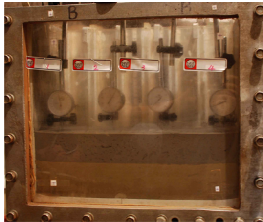
Fig. 7. Dial Gauge Installation Diagram
