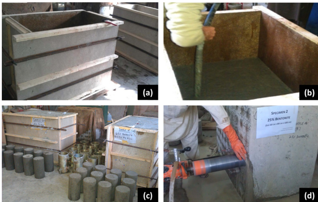
Fig. 4. Preparation of Mass Concrete Specimens
