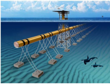
Fig. 4. Submerged Floating Railway Shaped as Pipe Line
