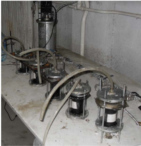
Fig. 6. Grouting Test Apparatus
