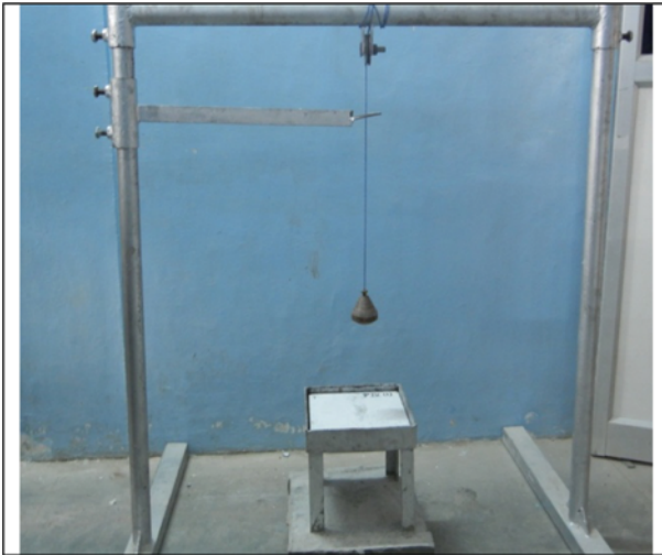
Fig. 2. Low-Velocity Impact Test Set-up
