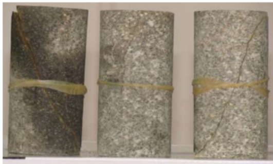
Fig. 3. Diabase Rock Samples after Shear Failure with Single Running-through Fracture
