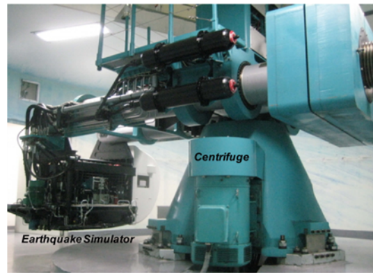
Fig. 1. Earthquake Simulator Mounted on the Centrifuge at KAIST
