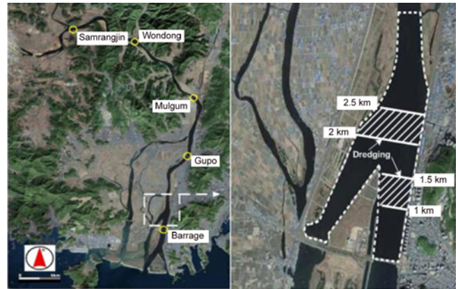
Fig. 4. 2D Modeling Section and Dredging Area in 2002 of the NREB
