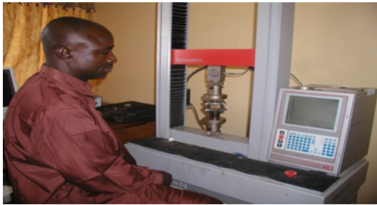
Fig. 5. Test Set-up for Compression Perpendicular to the Grain
