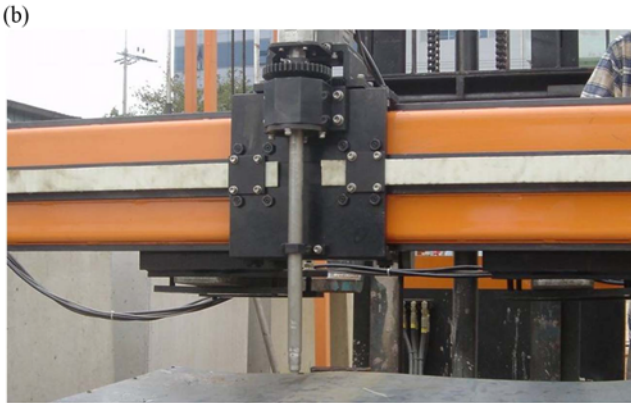
Fig. 2. Nozzle Guide System: (a) Schematic Diagram (unit: mm), (b) Photo of the Guide
