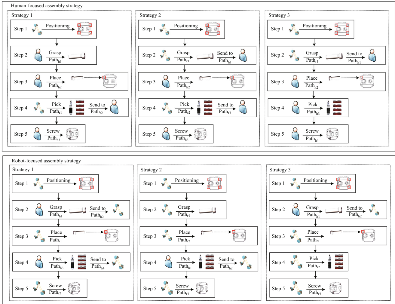
Fig. 5 Human-focused and robot-focused assembly strategies
