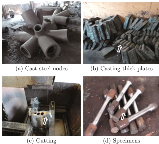
Fig. 1 Cast steel nodes and preparation of specimens
