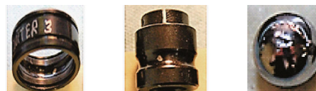
(a) Outer race (b) Inner race (c) Ball
