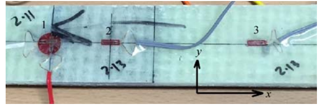
Fig. 4 Strain gauge locations on the sample surface (FBG sensor embedded between two layers and align with strain gauge 2 through the thickness)
