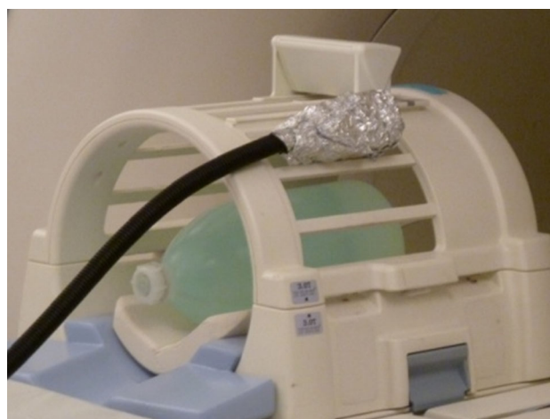
Fig. 4 RF head coil and the four-layer DOI detector
