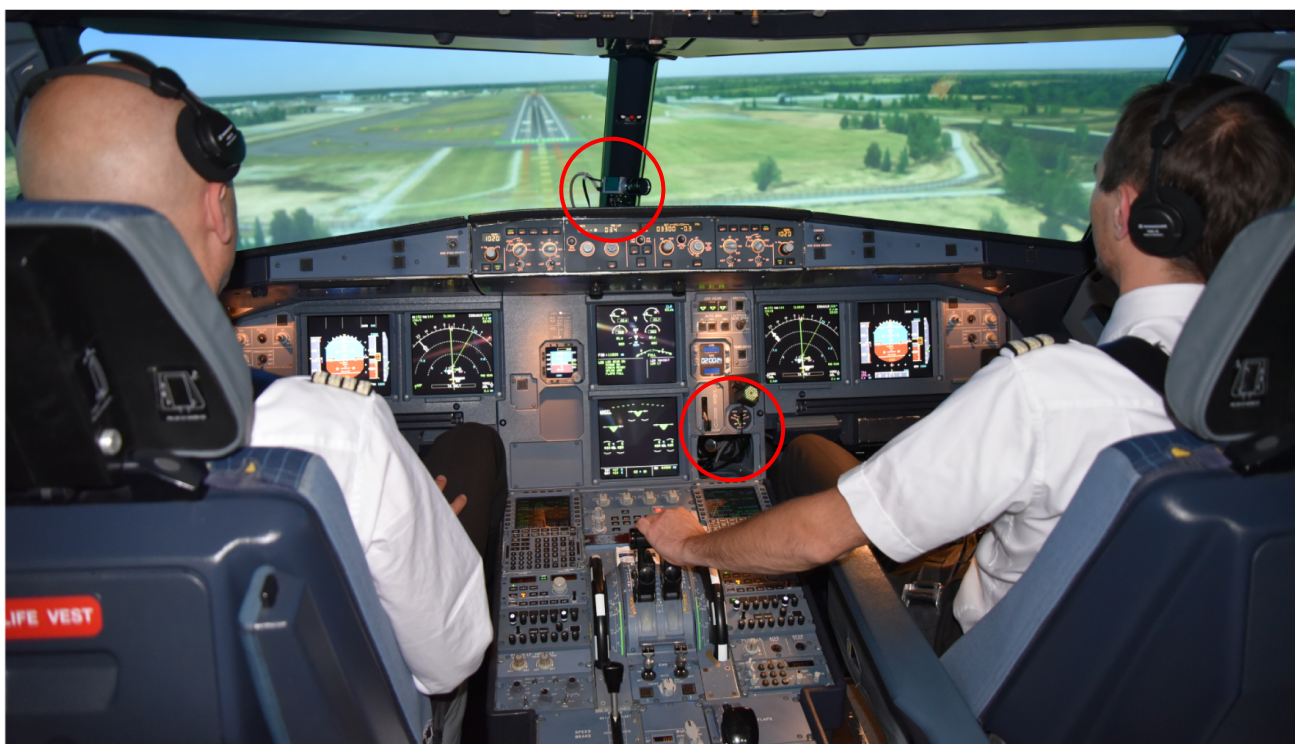
Fig. 2 Pilots in an A320 full flight simulator without a HUD. Also depicted is some of the eye tracking equipment (red circles, i.e., two cameras and one infrared emitter) that pilots had experience with (refer
